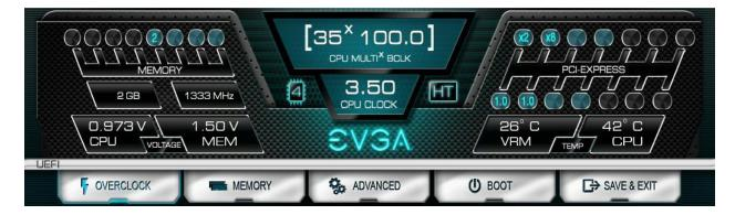
In the center above the EVGA logo, is basic CPU information. There is the overall CPU clock speed shown in GHz (Gigahertz). Above that the CPU Multiplier times Base Clock (BCLK) which is how clock speed is derived. Adjacent to the CPU Clock there is a small outline of a chip and a number inside of it, the number in this case 4, is the number of physical cores in the CPU. HT indicates that Hyper Threading is enabled.
