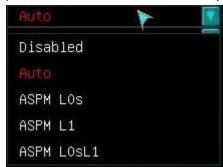
Disable/Auto/ASPM (Active State Power Management) L0s/ASPM L1/ASPM L0sL1 Disable – Removes ASPM support for this PCI-e slot.
