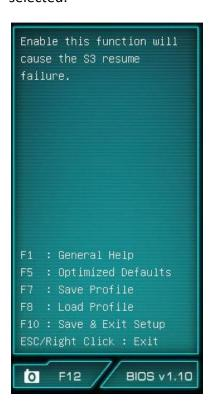
The upper portion will give you a brief explanation of a selected item. Below that are the basic commands for the BIOS. The modern UEFI (Unified Extensible Firmware Interface) BIOS GUI also allows for full navigation via mouse or the arrow keys.
