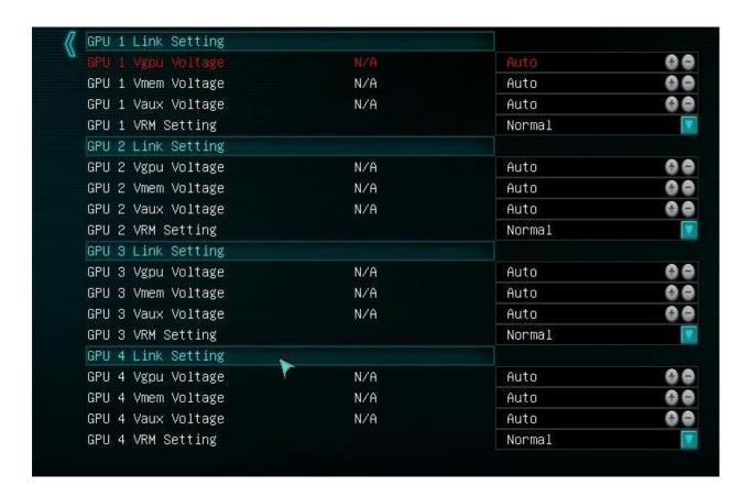
There are 4 GPU link settings, all options and ranges are identical, this is strictly for adjusting up to 4 video cards individually.
